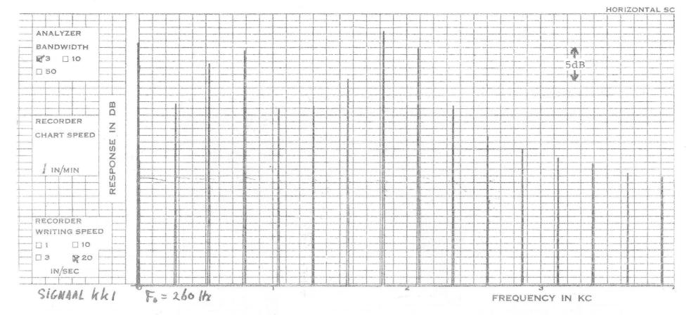
Fig.8 Spectrum of signal KK1,  $F_0 = 260$ Hz,  $F_1 = 700$ Hz,  $F_2 = 1950$ Hz
