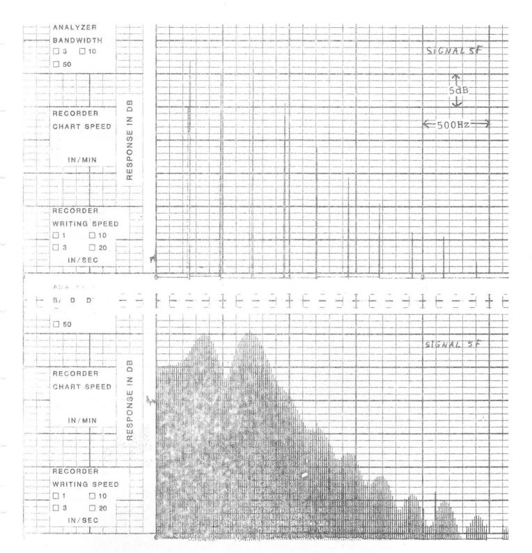
Fig.11 Spectrum of signal 5F,  $F_0 = 240$ Hz,  $F_1 = 400$ Hz,  $F_2 = 700$ Hz Fig.11a Spectrum of signal 5F with time-insertion,  $F'_0 = 14.4$ Hz
