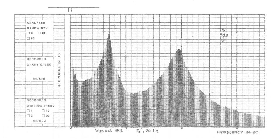
Fig.8a Spectrum of the signal from fig.8 with time-insertion, F'=20Hz
