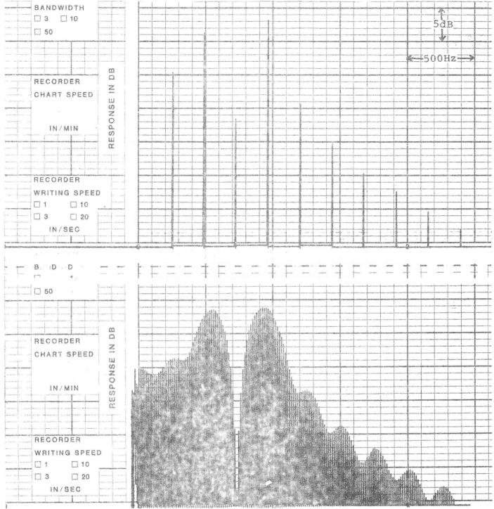
Fig.13 Spectrum of signal 7F,  $F_0 = 240$ Hz,  $F_1 = 580$ Hz,  $F_2 = 930$ Hz Fig.13a Spectrum of signal 7F with time-insertion,  $F_0^{!=14.4Hz}$
