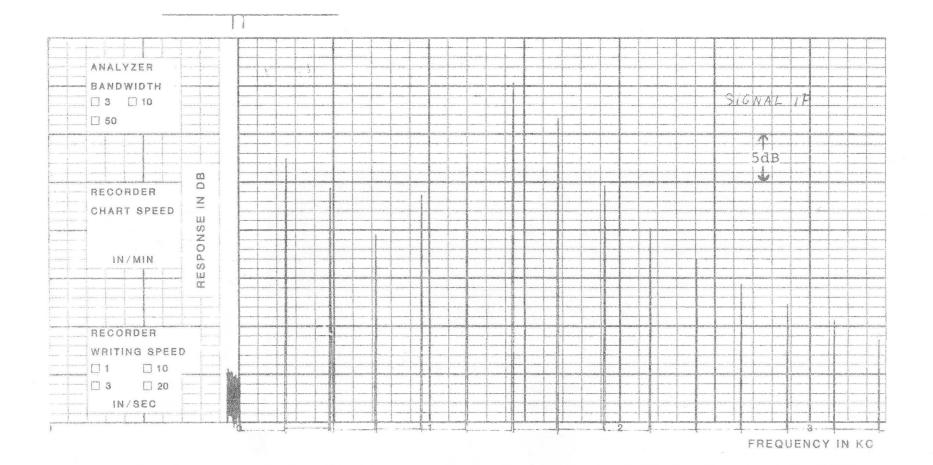
Fig.10 Spectrum of signal 1F,  $F_0 = 240$ Hz,  $F_1 = 400$ Hz,  $F_2 = 1500$ Hz
