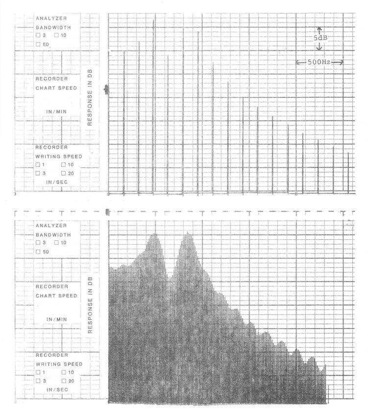
Fig.12 Spectrum of signal 2M,  $F_0 = 160$ Hz,  $F_1 = 540$ Hz,  $F_2 = 860$ Hz Fig.12a Spectrum of signal 2M with time-insertion,  $F'_0 = 14.4$ Hz
