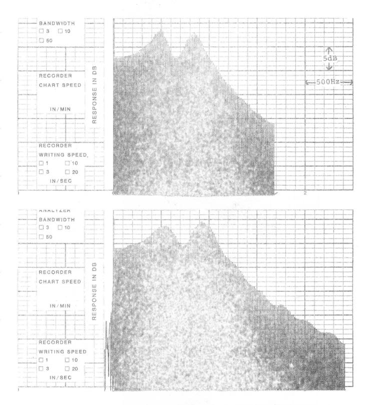
Fig.15 Spectrum of the signal from fig.12 (signal 2M) with timeinsertion and exponential window multiplication,  $\alpha_a \approx 200$ Fig.16 Spectrum of the signal from fig.13 (signal 7F) with timeinsertion and exponential window multiplication,  $\alpha_a \approx 350$
