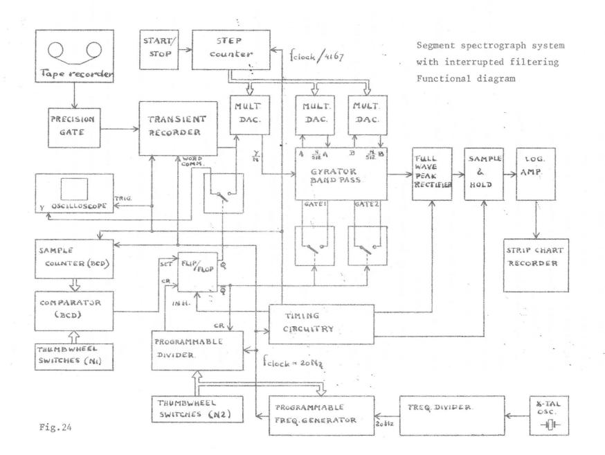
transient recorder is attenuated by a digitally controllable divider (using a multiplying digital-to-analog convertor) and then led to the input of the gyrator band pass filter.
